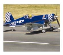
to fleet carriers in ever increasing numbers. The F4U had an inverted gull wing, a streamlined fuselage of circular cross-section and a large propeller. The cockpit was set well back, and the restricted view required careful handling by the skilled pilots flying the aircraft.
